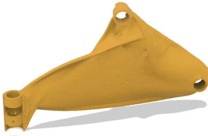
Figure 43: Updated Generative Design for Back Truss
