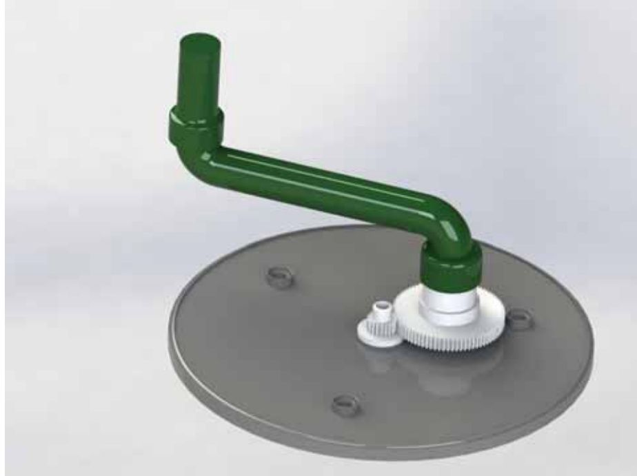
Figure 21: Lid Gearing Assembly
