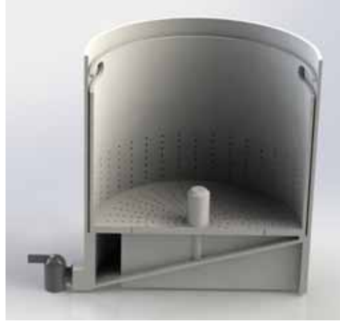
Figure 47: Cutaway of Inner Pot Resting on Ribs (Angle Increased to 15 Degrees for Clarity)
