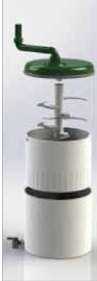
Figure 49: Full Assembly Showing Removing the Center Pot and Blade Assembly
