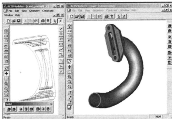
(a) engine case data accessible for exhaust manifold designer
