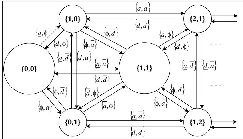
Figure 4-11:  $[M]/[M]/1$  queueing system state transition diagram
