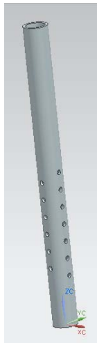
Figure 20b. Bottom Outer Shin Pipe Final.
