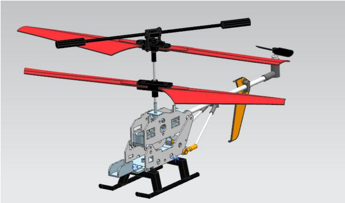
Redesigned Structural Design Assembly
