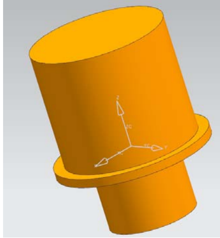
Figure 31: Barrel tip – revolve
