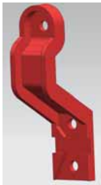
(g) Bolt Holes Established
